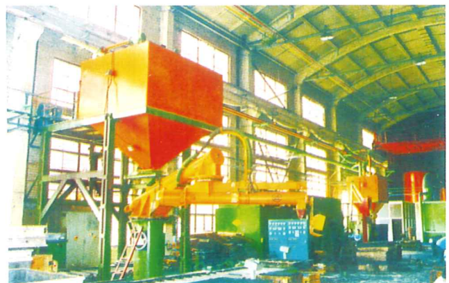
图02德国树脂砂造形生产线 Fig.02 The Resin Sand Mold Production Line Made in Germany
